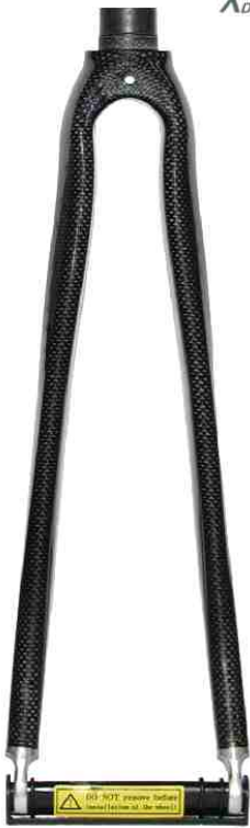
FF4 - Carbon Fork Monocoque 700C. 25.4mm Non Integrated. 43mm Offset. Raked. 365 g Av. FF8 - Carbon Fork Monocoque 700C. 28.6mm Integrated. 43mm Offset. Raked. 395 g Average.
