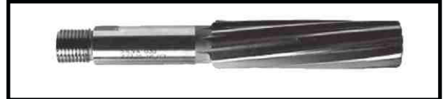
Art. 30. Seat Tube Reamer Diameter 27.2mm.
