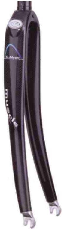
Muscle - 28.6mm Integrated. Monocoque Fork With Titanium Mesh. 45mm offset. 300mm Carbon Steerer. 380g Average. Super Muscle - Same Shape as above. 28.6mm Integrated. Monocoque Fork with Nickel Braiding. 45mm Offset. 300mm Carbon Steerer. 340g Average
